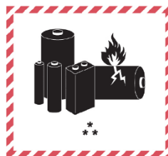
Figure 3: Lithium battery identification
