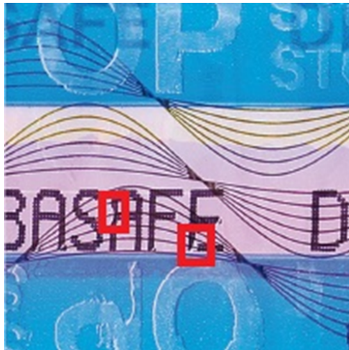
Figure 12 : Example 1 for a damaged black security overprint
