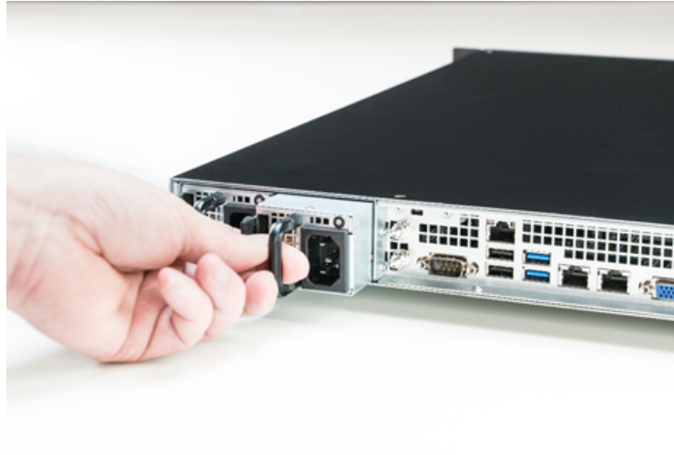
Figure 62 : Using the power supply handle
