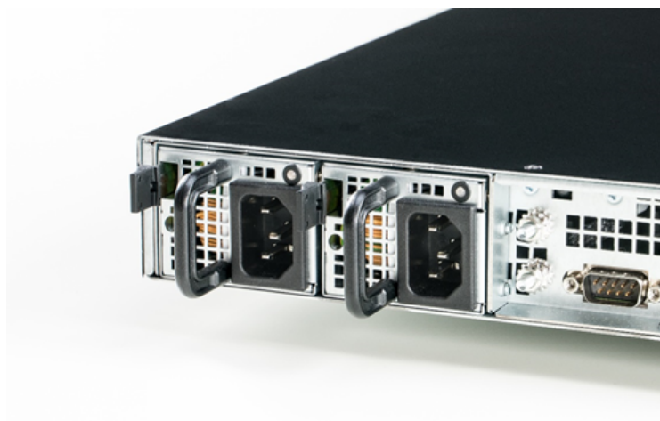
Figure 60 : The power supply modules on the rear side of the u.trust Anchor LAN V5
