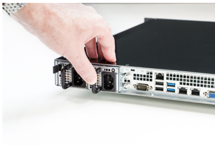
Figure 65 : Pressing the handle of the new power supply module
