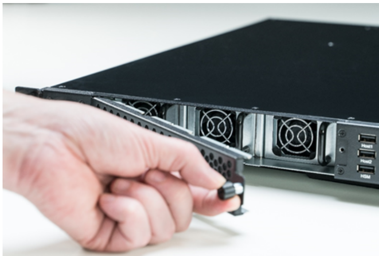
Figure 67 : Opening the fan compartment
