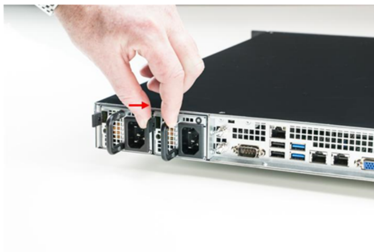
Figure 61 : Pressing the locking of a power supply module
