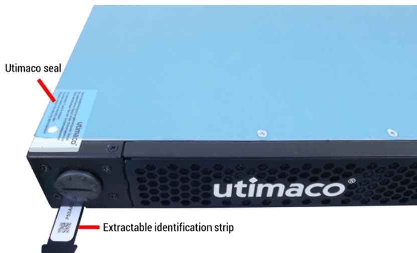
Figure 19 : Extractable identification strip on the u.trust Anchor LAN
