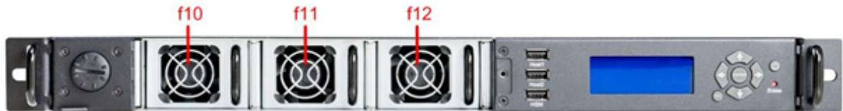
Figure 50 : u.trust Anchor LAN V5 – Front panel with removed fan compartment grill
