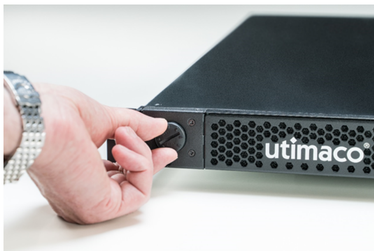
Figure 54 : Turning the screw cap of the battery compartment of the u.trust Anchor LAN V5
