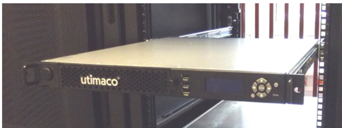
Figure 75 : u.trust Anchor LAN V5 in the locked position
