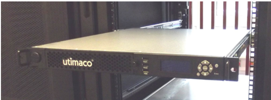
Figure 36 : u.trust Anchor LAN V5 in the locked position
