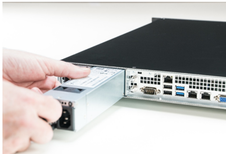
Figure 63 : Pulling the power supply module out of the case
