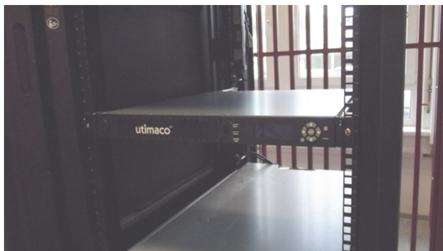
Figure 39 : u.trust Anchor LAN V5 mounted on a rack
