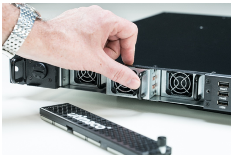
Figure 69 : Putting the new fan module in place
