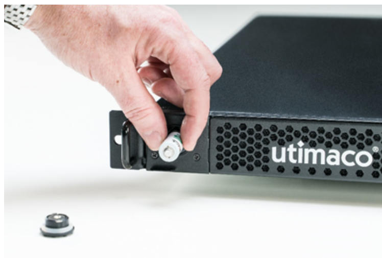
Figure 57 : Removing the external battery of the u.trust Anchor LAN V5
