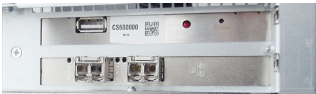
Figure 44 : Optical fiber network interface card without dummy plugs
