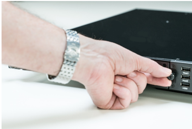
Figure 66 : Turning the knurled screw
