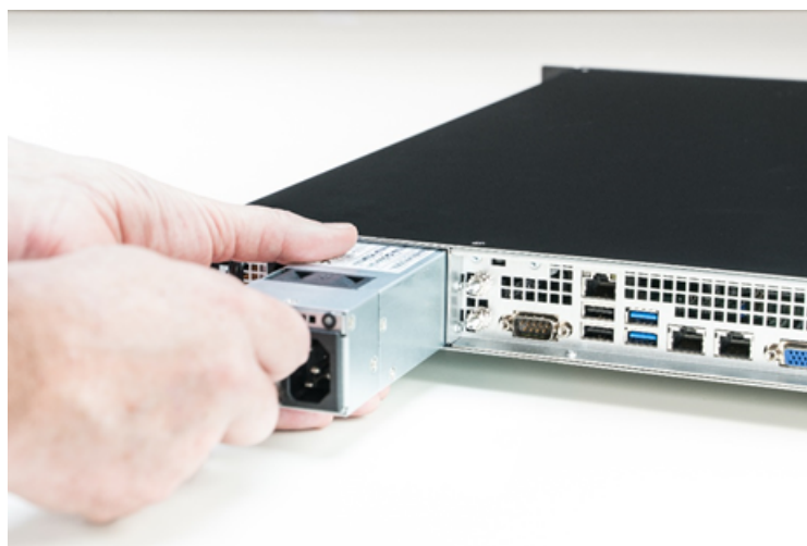
Figure 64 : Putting the new power supply module in place
