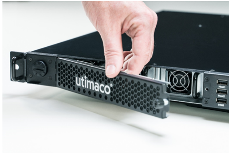
Figure 70 : Placing the cover
