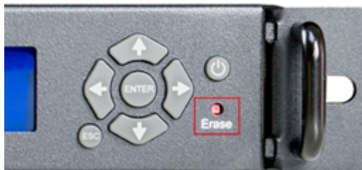
Figure 71 : ERASE push-button for performing External Erase on a u.trust Anchor LAN V5
