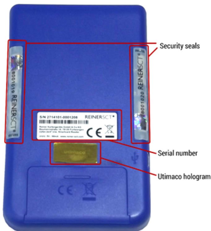
Figure 21 : Serial number and Security seals of the PIN pad
