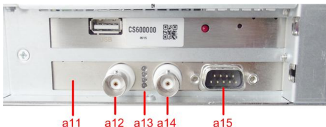
Figure 42 : PCIe clock card on the rear side of u.trust Anchor LAN V5
