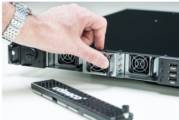
Figure 69 : Putting the new fan module in place
