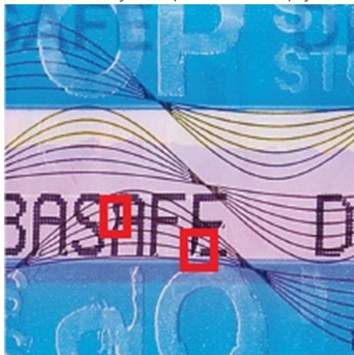
Figure 12 : Example 1 for a damaged black security overprint
