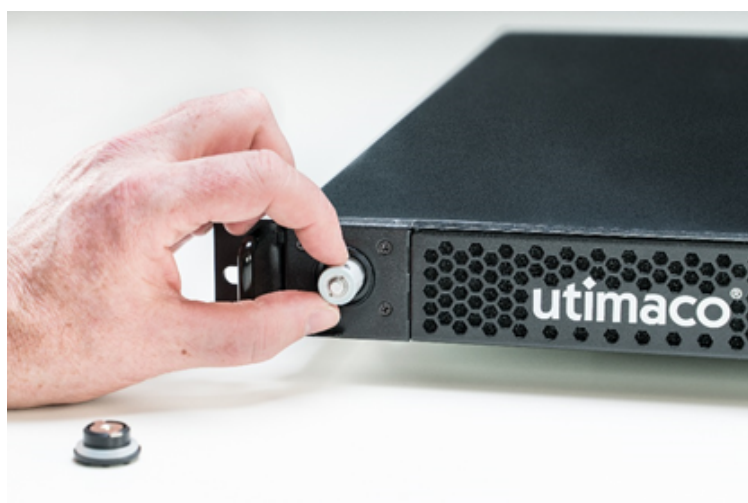
Figure 58 : Placing the new battery in the battery compartment
