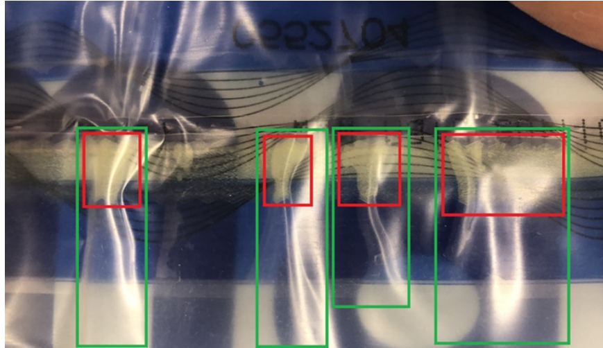
Figure 7 : Example for acceptable yellow spots and folds
