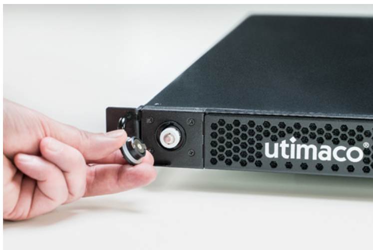
Figure 56 : Removing the screw cap of the battery compartment
