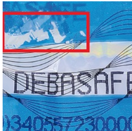
Figure 16 : Example 2 for a damaged blue stripe
