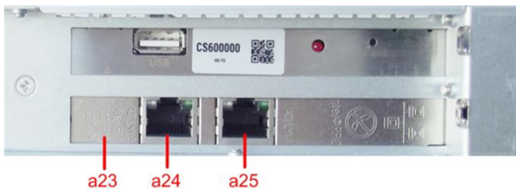
Figure 47 : Copper network interface card on the rear side of u.trust Anchor LAN V5
