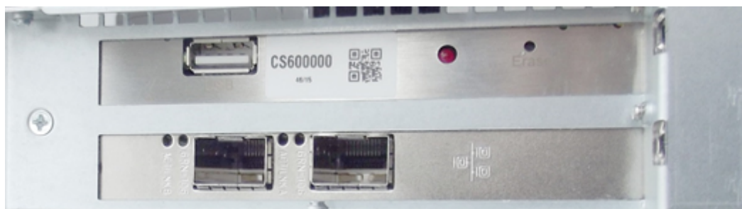
Figure 45 : Optical fiber network interface card without SFP transceiver modules
