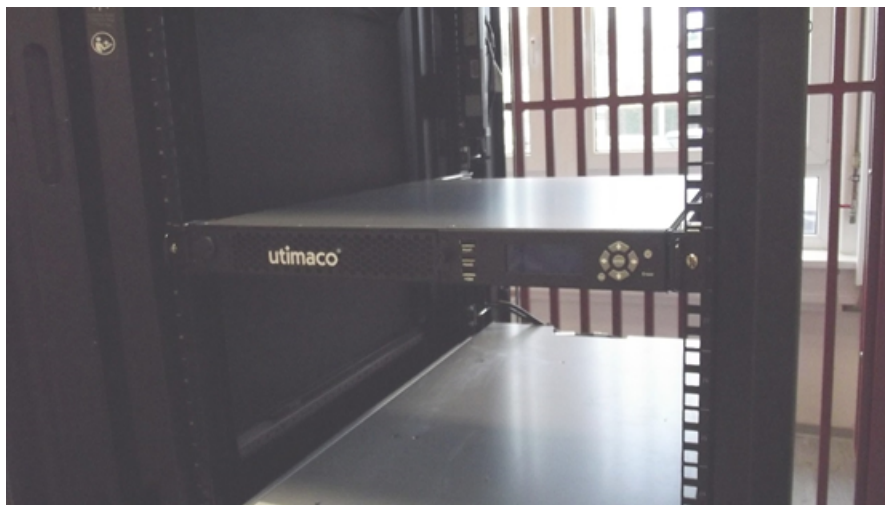
Figure 73 : u.trust Anchor LAN V5 mounted on a rack
