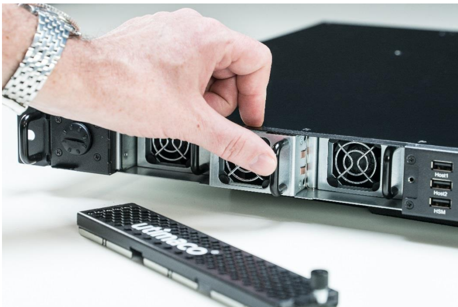
Figure 51: Putting the new fan module in place
