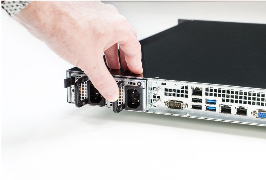
Figure 47: Pressing the handle of the new power supply module
