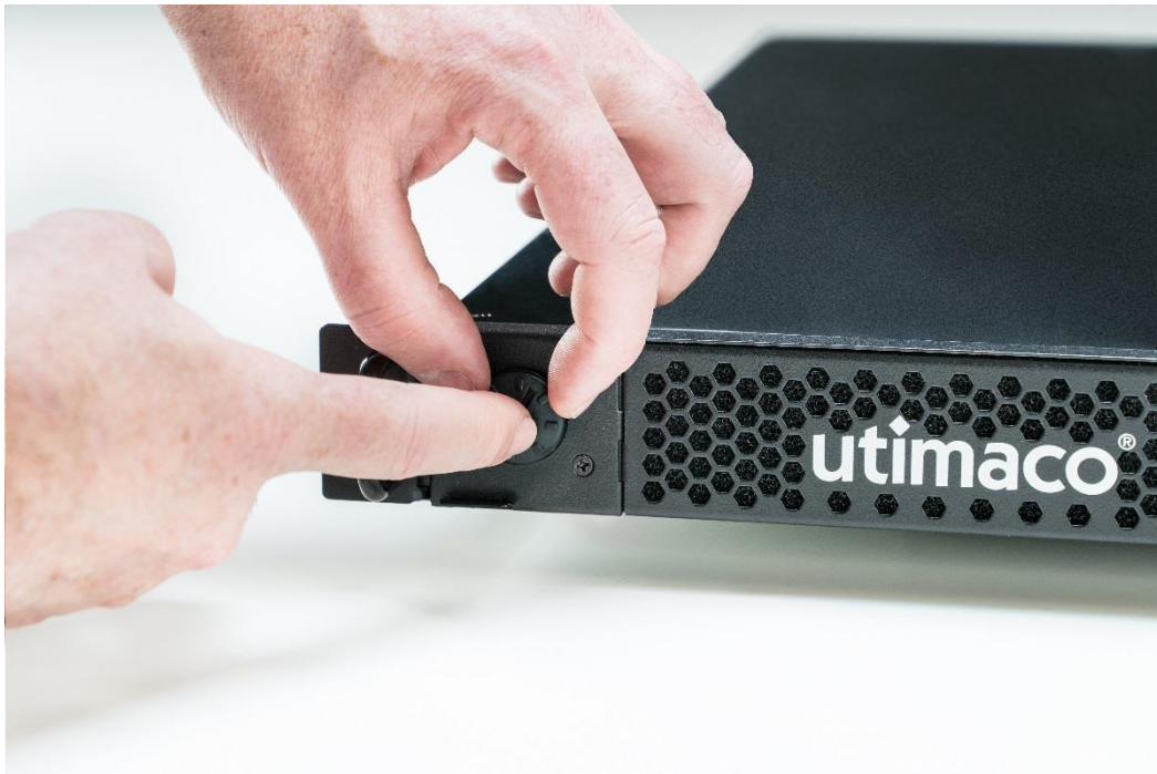
Figure 41: Screwing on the screw cap of the battery compartment for the external battery
