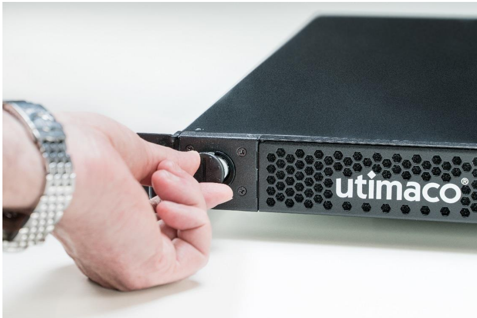
Figure 37: Opening the battery compartment of the CryptoServer LAN V5
