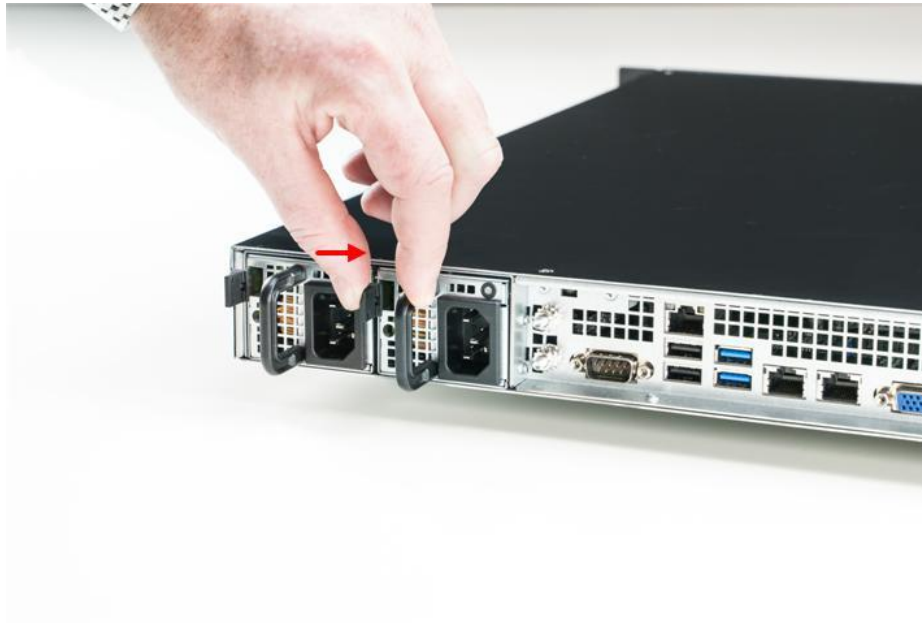
Figure 43: Pressing the locking of a power supply module
