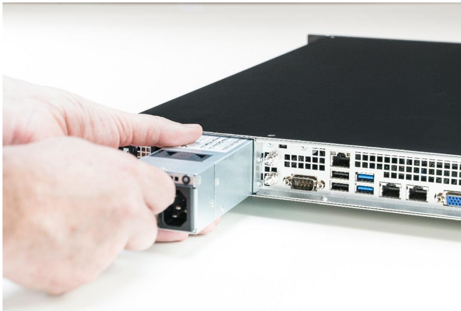
Figure 46: Putting the new power supply module in place
