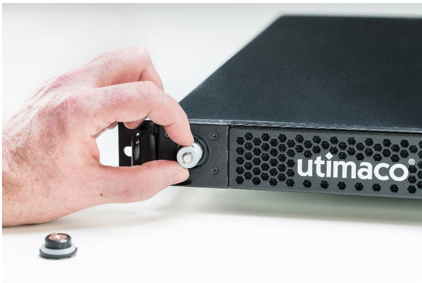
Figure 40: Placing the new battery in the battery compartment
