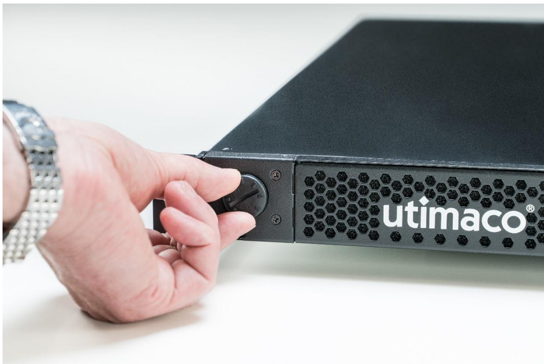
Figure 36: Turning the screw cap of the battery compartment of the CryptoServer LAN V5
