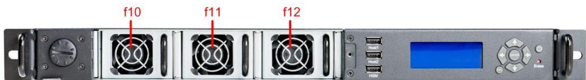
Figure 32: CryptoServer LAN V5 – Front panel with removed fan compartment grill
