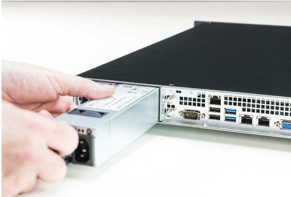
Figure 45: Pulling the power supply module out of the case
