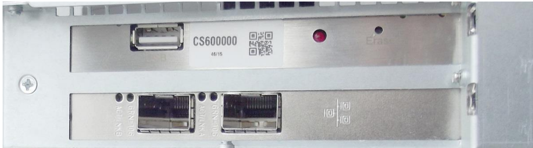
Figure 27: Optical fiber network interface card without SFP transceiver modules
