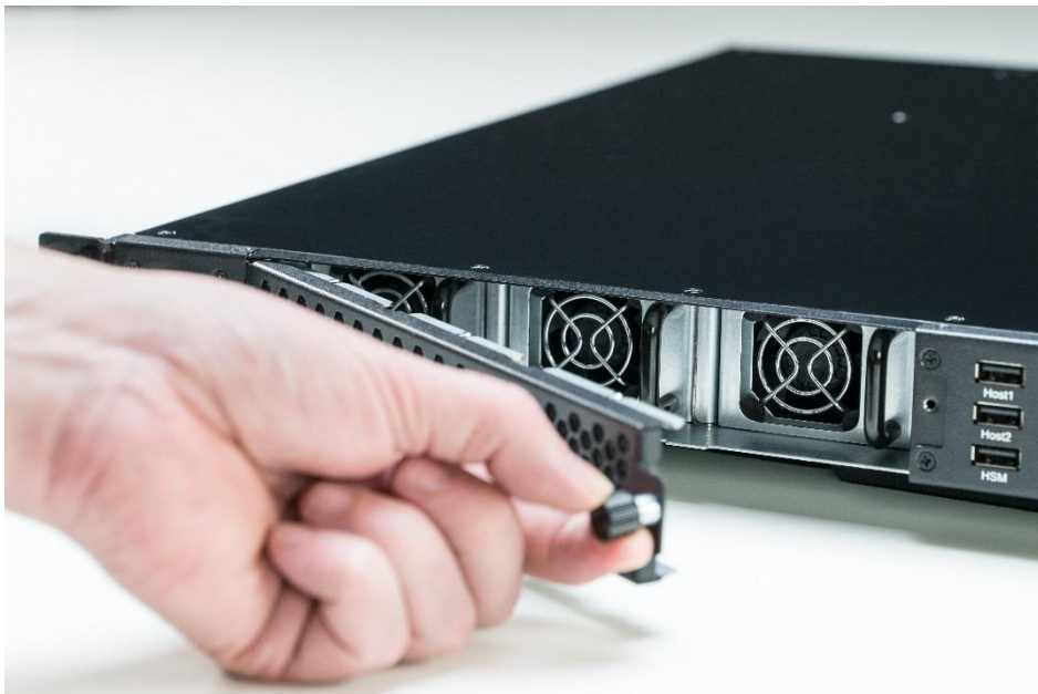
Figure 49: Opening the fan compartment
