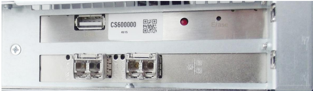
Figure 26: Optical fiber network interface card without dummy plugs
