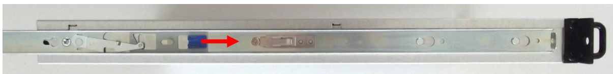
Figure 16: Pulling the pin-lock latch on the left side of the CryptoServer LAN V5
