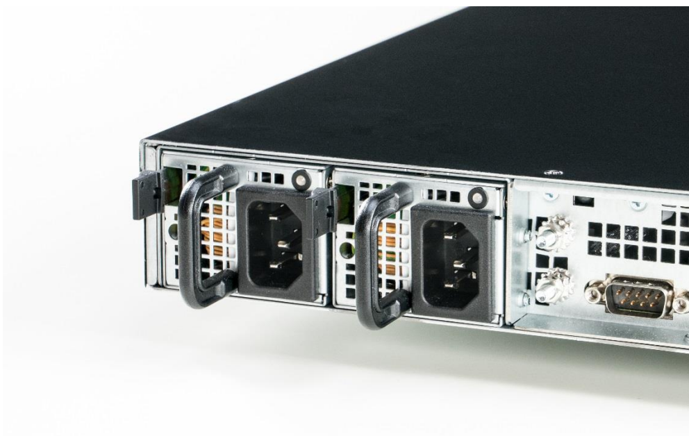
Figure 42: The power supply modules on the rear side of the CryptoServer LAN V5
