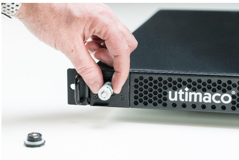
Figure 39: Removing the external battery of the CryptoServer LAN V5
