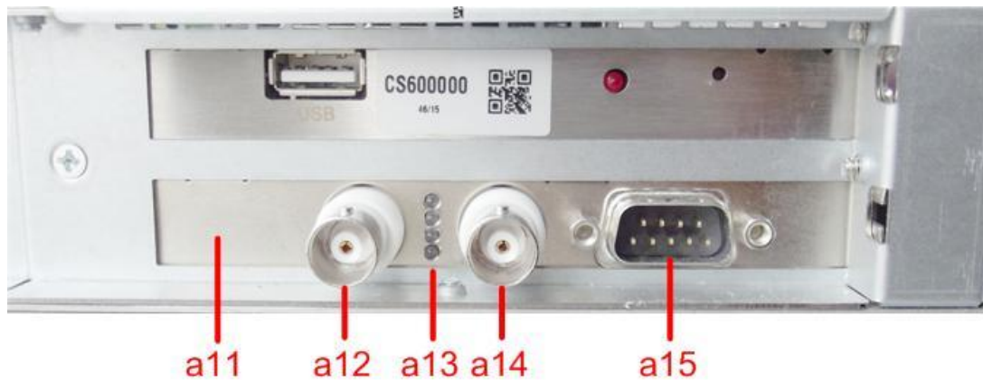
Figure 24: PCIe clock card on the rear side of CryptoServer LAN V5
