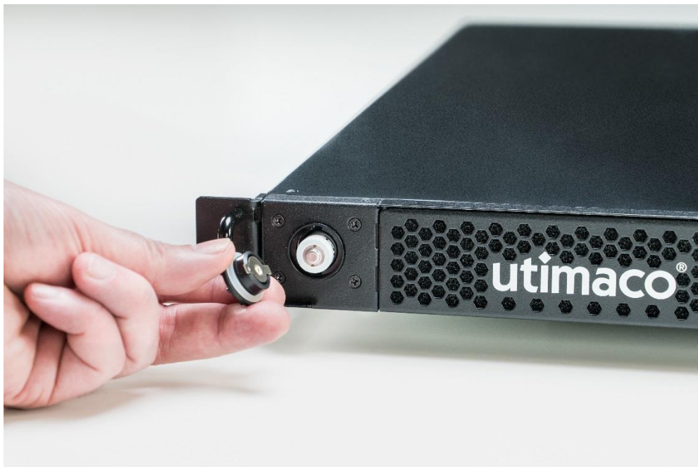
Figure 38: Removing the screw cap of the battery compartment
