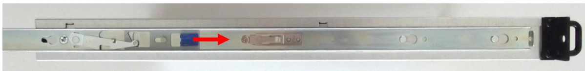
Figure 58: Releasing the pin-lock latch on the left side of the CryptoServer LAN V5
