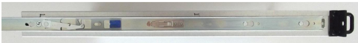
Figure 14: Inner slide rail mounted on the CryptoServer LAN V5
