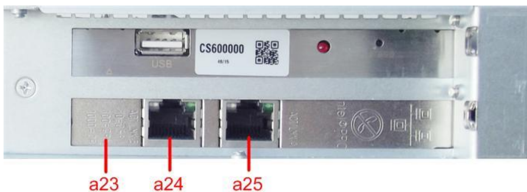
Figure 29: Copper network interface card on the rear side of CryptoServer LAN V5
