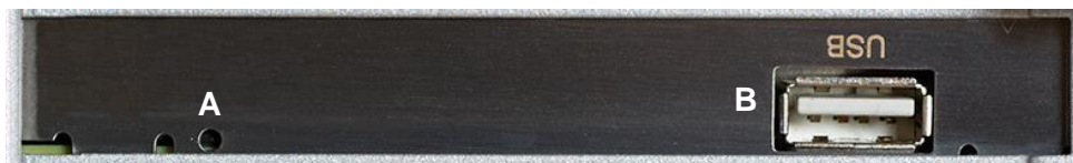
Figure 21: CryptoServer CSe – Sockets and ports on the rear side
