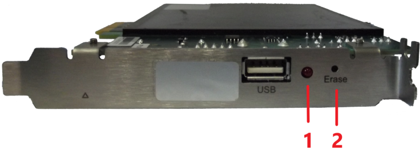
Figure 18 : u.trust Anchor PCIe card - slot plate
