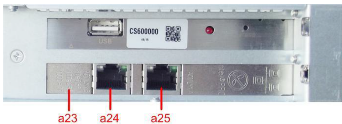
Figure 12 : Optional Copper Network Interface Card on the Rear Side
