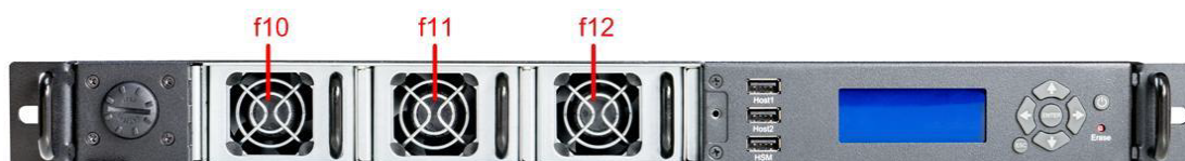
Figure 32 : Front panel with removed fan compartment grill
