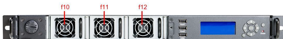
Figure 32 : Front panel with removed fan compartment grill
