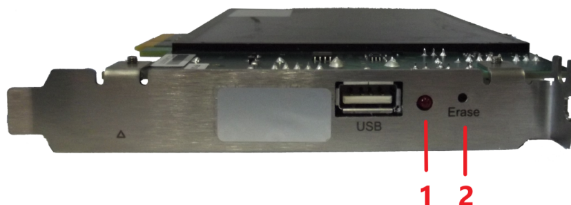
Figure 20 : u.trust Anchor PCIe card - slot plate
