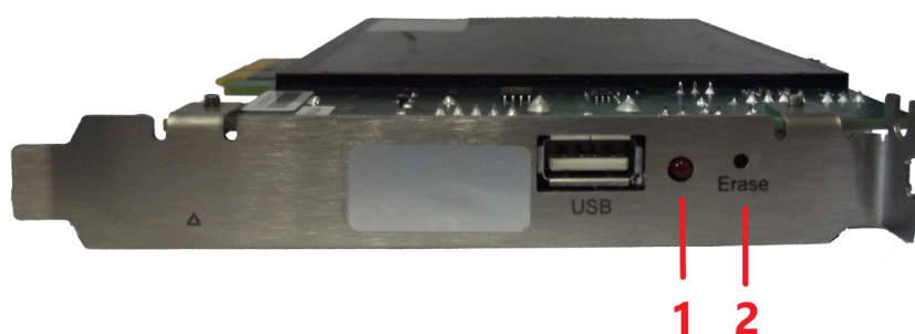
Figure 18 : u.trust Anchor PCIe card - slot plate
