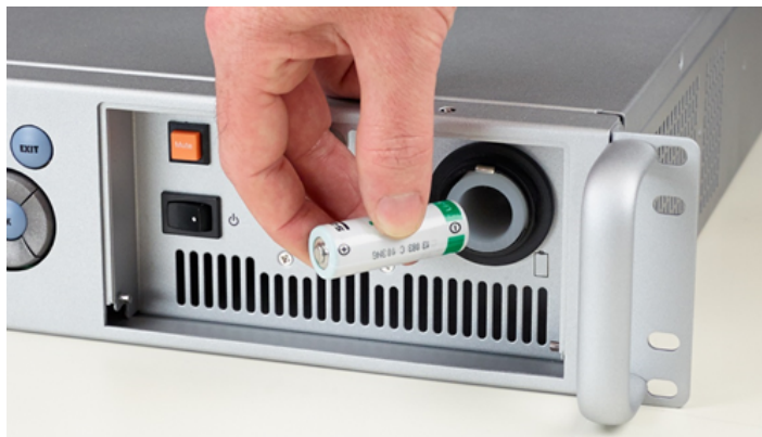
Figure 38 : The external battery of the CryptoServer LAN V4
