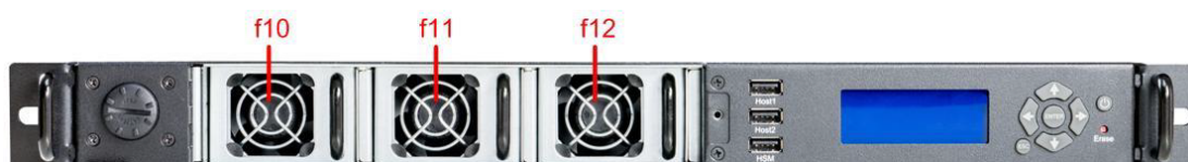
Figure 10 : Front panel with removed fan compartment grill
