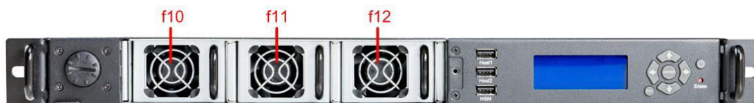
Figure 22 : Front panel with removed fan compartment grill
